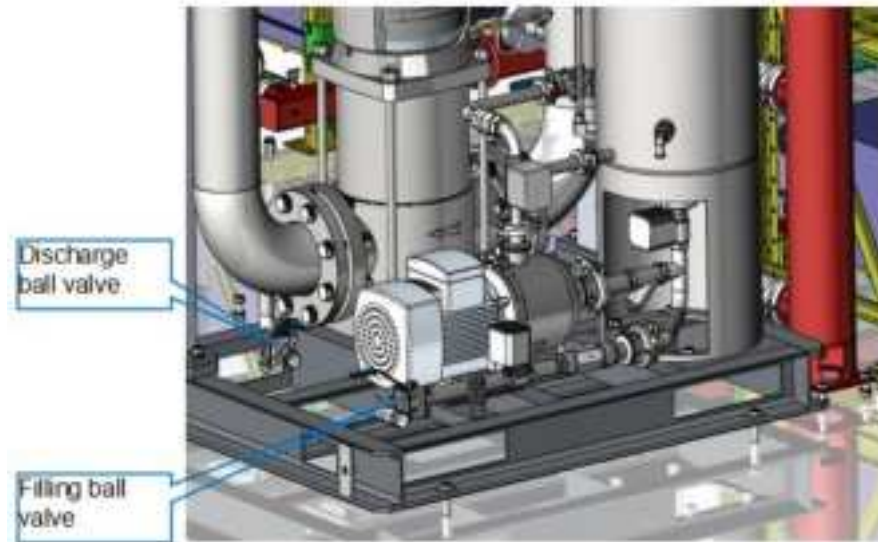
Figure 10-25 Location of discharge ball valve in pump station
