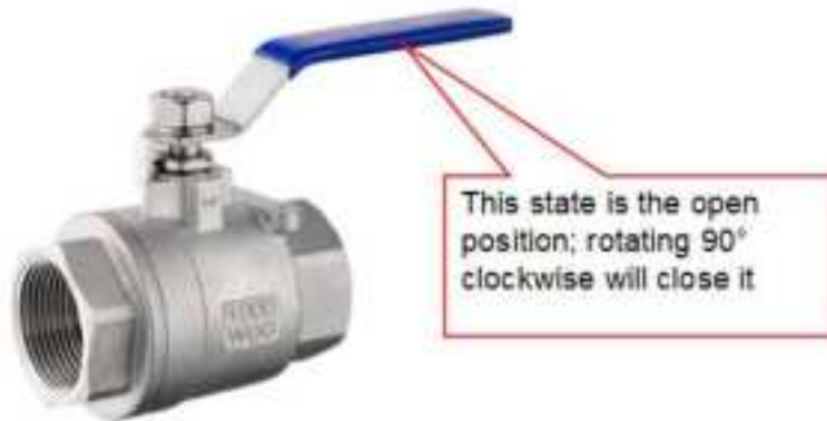
Figure 8-15 Schematic diagram of valve opening and closing
