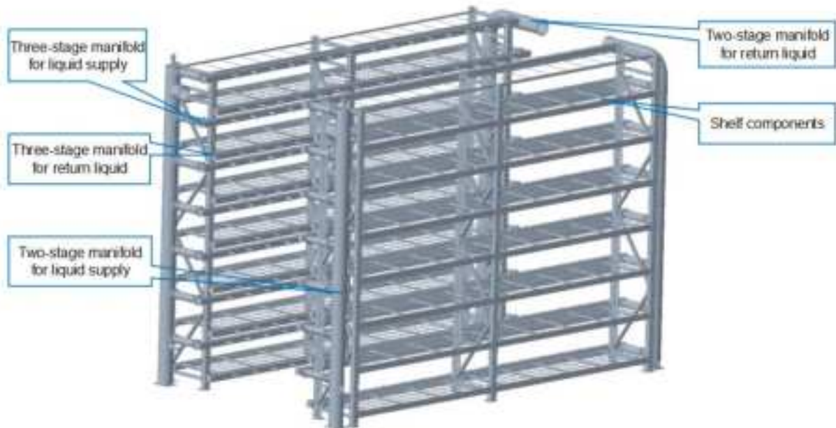
Figure 5-5 Internal view of manifold components
