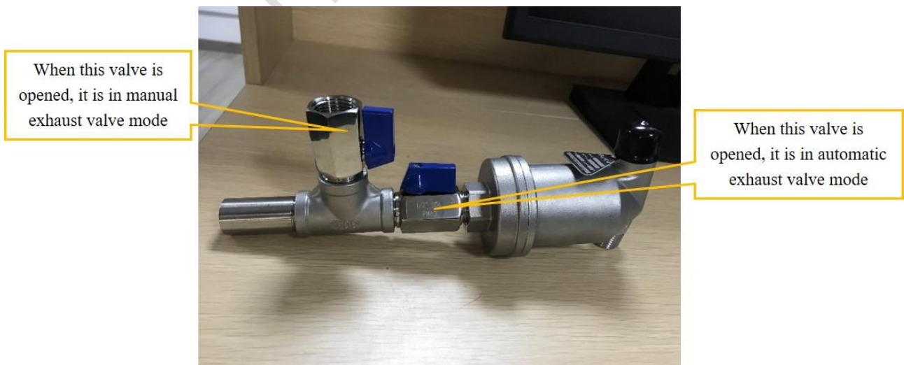
Figure 7.14 Dry tower exhaust valve.
