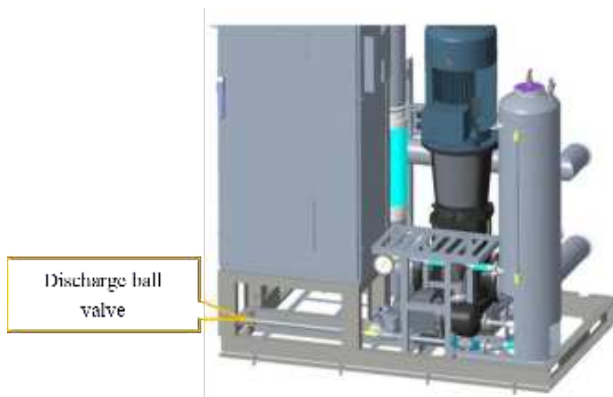
Figure 9.3 Location of discharge ball valve in pump station.
