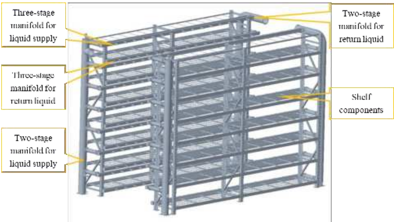
Figure 5.4 Internal view of manifold components.
