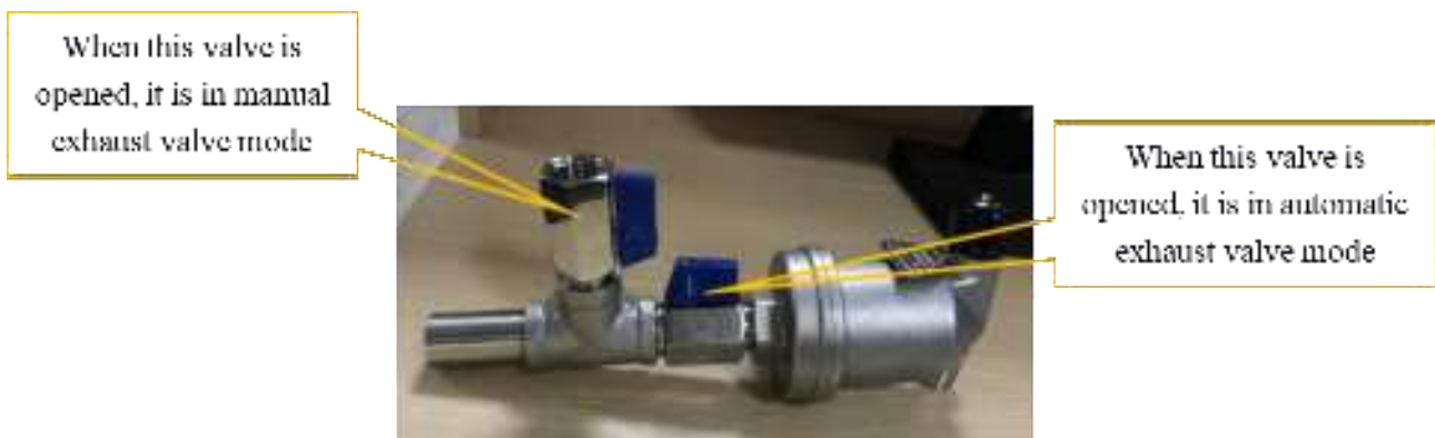
Figure 7.13 PHE exhaust valve.
