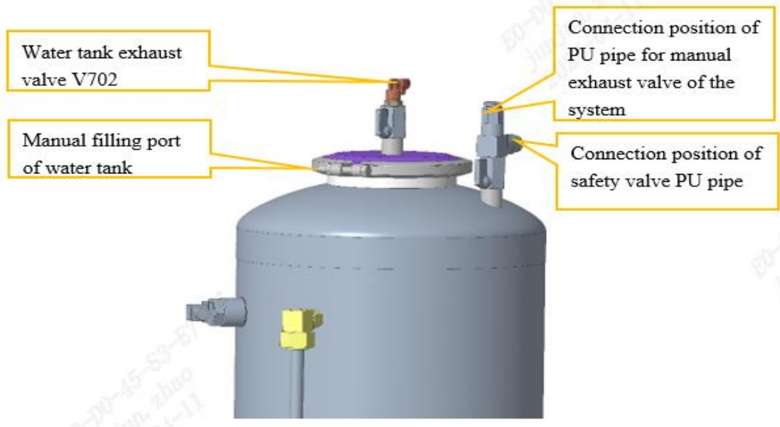
Figure 7-12 Water tank valve
