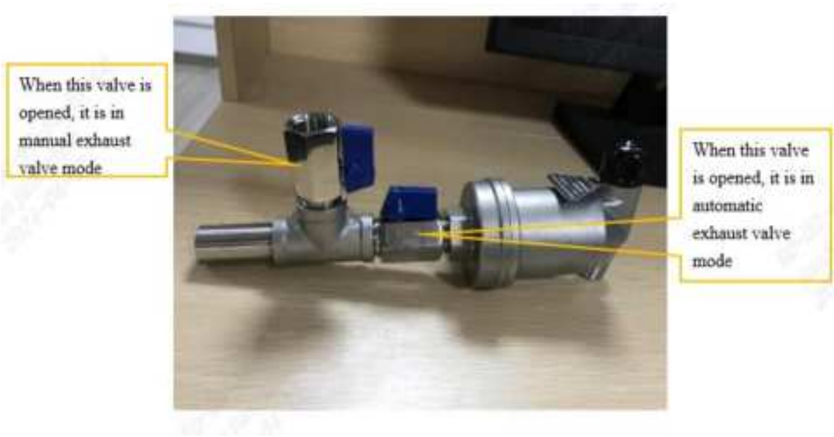
Figure 7-13 Cooling tower exhaust valve
