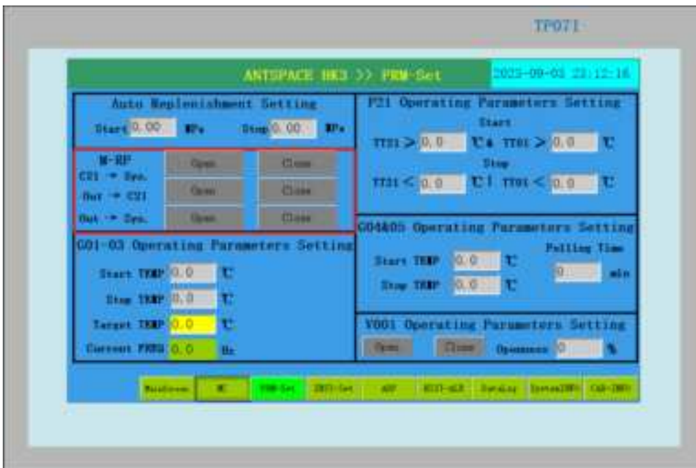
Figure 7-15 Water filling system interface
