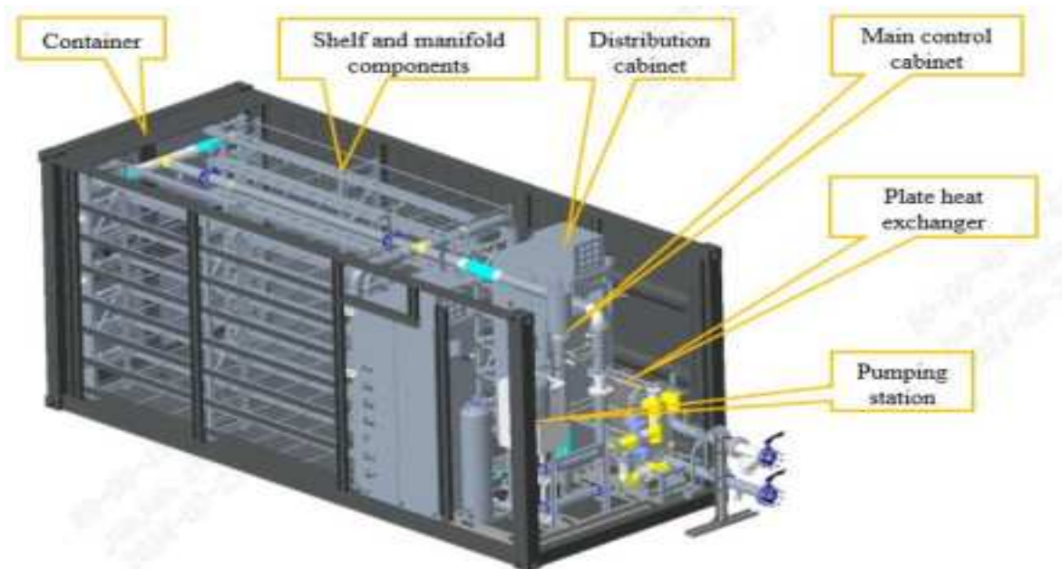
Figure 5-2 Internal view of container
