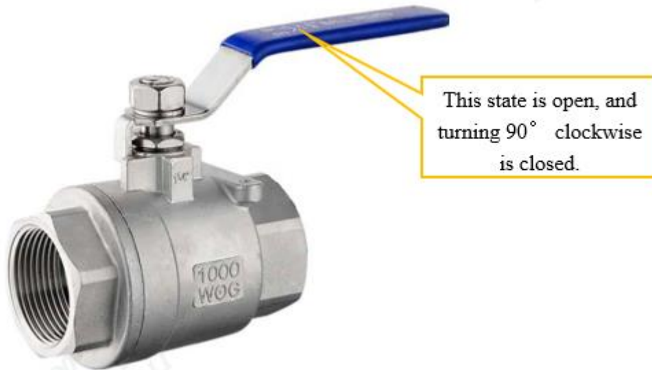
Figure 7-7 Schematic diagram of valve opening and closing
