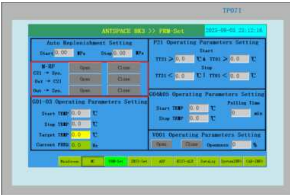
Figure 7-15 Liquid filling system interface
