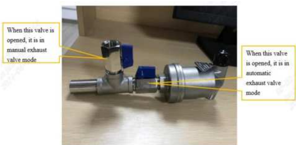
Figure 7-13 Dry tower exhaust valve
