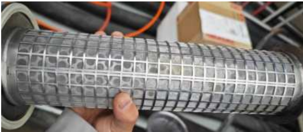
Figure 9-2 Remove the pipeline filter
