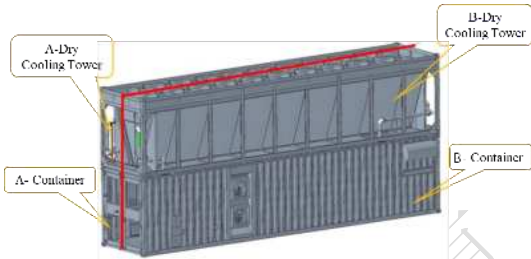
Figure 6.10 Schematic diagram of the dry cooling tower with the AB side of the container. (split by the red center line)
