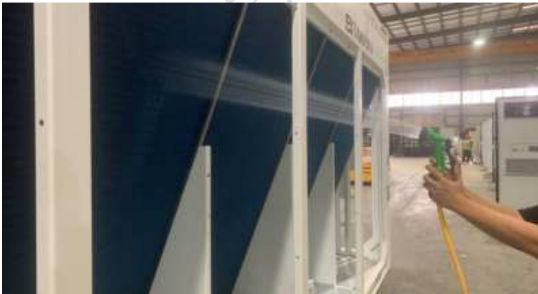
Figure 9.5 Schematic diagram of cleaning heat exchanger fins
