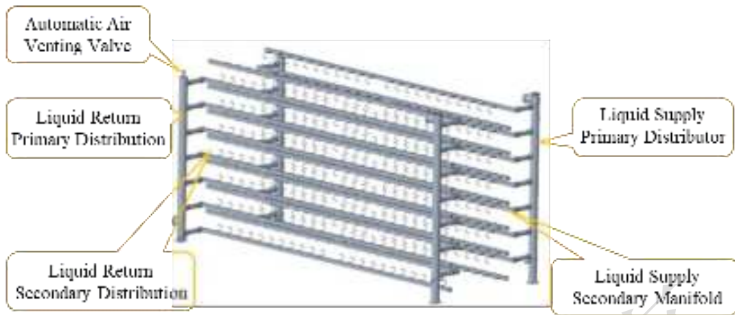
Figure 5.3 Internal view of manifold assembly
